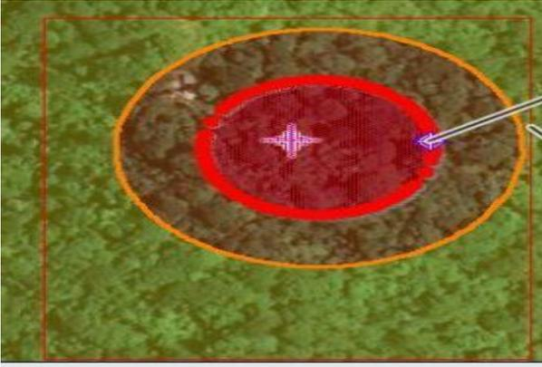
**Fig. 12:** Footprint of VCE from H<sub>2</sub>, Plant 2–day, 25 mm leakage, 15% fatalities (from WNW wind direction).
