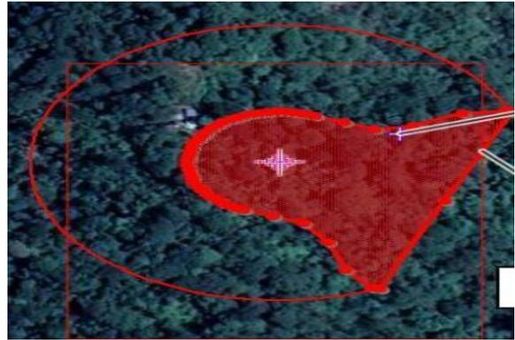
**Fig. 4:** Puff dispersion at Plant 1–release of CO<sub>2</sub> at night, 160 mm leakage, 27% fatalities (from WNW wind direction).
